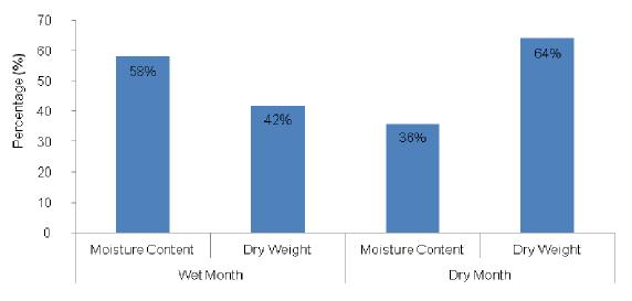
Figure 4. Wet and dry month moisture content and dry weigh of the soild waste.
