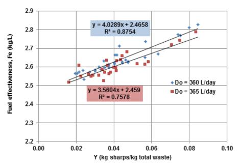
Figure 6. Effect of sharps waste proportion on fuel effectiveness during incineration of infectious medical waste.
