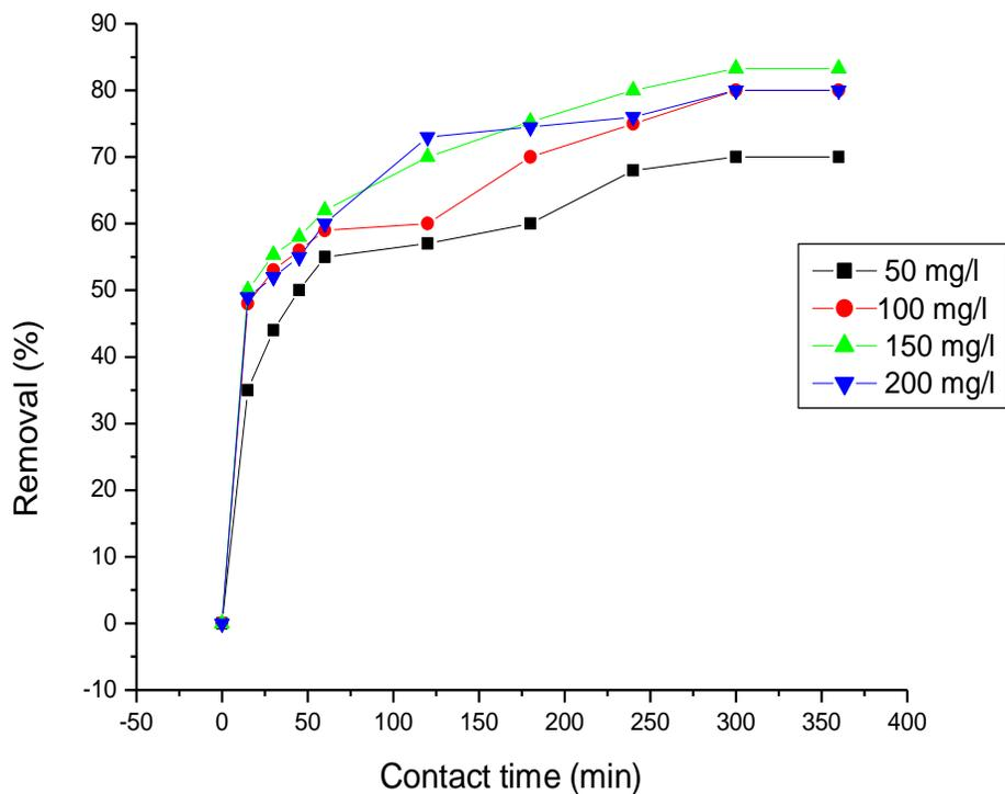
**Figure 8.** Removal of irgalite by *P. putida* at various initial concentrations in the reaction mixtures. AC dose was 8gm/l. Initial concentration= 50, 100, 150 and 200 mg/L, pH 7.
