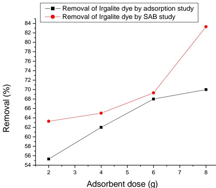
**Figure 6.** Comparison Effect of adsorbent dose on %removal of irgalite dye between adsorption and SAB study at conc. 150 mg/l, ph 7.
