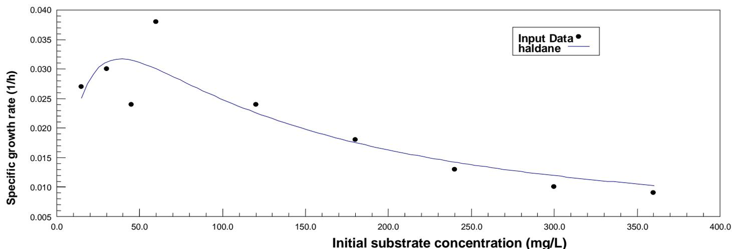
**Figure 4.** Biodegradation kinetics (Haldane's model) for free *P. putida* for initial concentration ranging from 10 to 350 mg irgalite/l in the reaction mixture.
