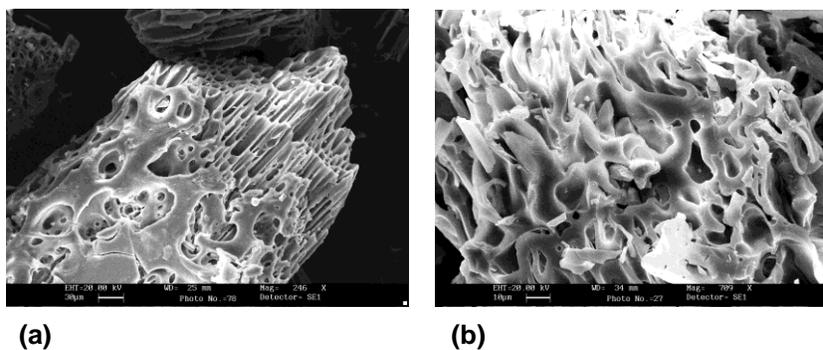
**Figure 10.** (A) Adsorption study .Scanning electron micrograph of 2 to 4 mm carbon particles at 1000x magnification after adsorption of irgalite; (B), SAB study. Scanning electron micrograph of 2 to 4 mm, carbon particles at 1000x magnification after, SAB of irgalite
