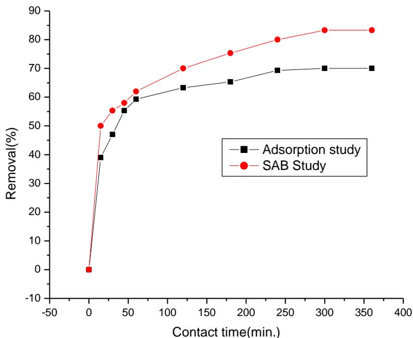
**Figure 9.** Comparison of dye removal by simple adsorption and SAB. For both the experiments initial concentration of irgalite dye was 50 mg /l in the reaction mixture. AC dose was 8 mg/l. For SAB 20 ml *P. putida* inoculums was used. SAB and adsorption.
