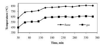
Figure 3. Flame and producer gas temperature.
