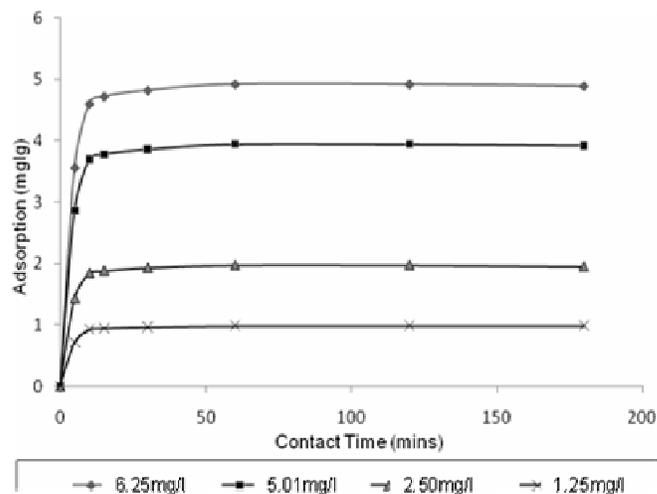
Figure 2. Adsorption rate of Cr<sup>6+</sup> onto PAC at different initial Cr<sup>6+</sup> concentrations for the flocculation effluent of LP-OBDC.
