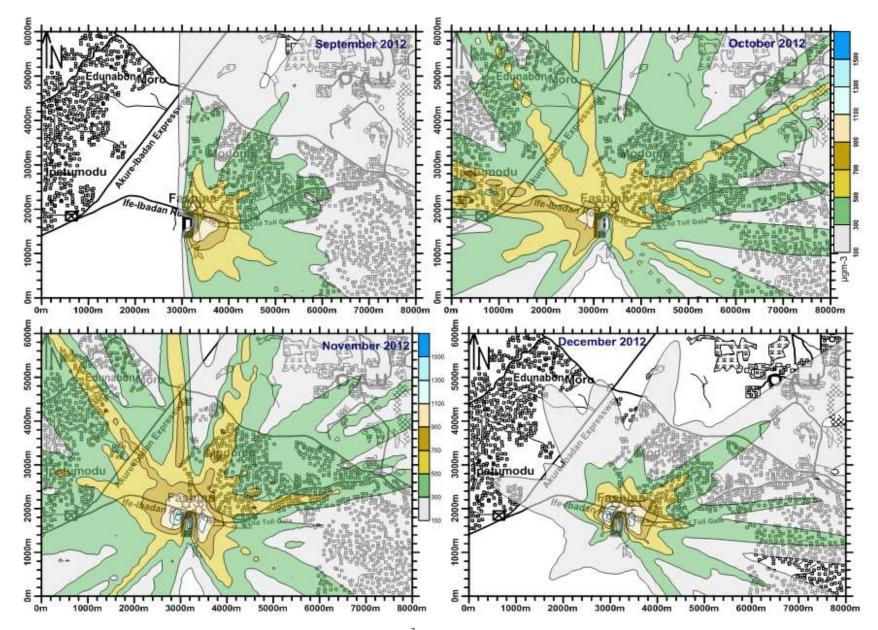
Figure 3. Ventilation corridors and concentration spread (color scale in µgm<sup>-3</sup>) for CO in the months of Sepetember (top left), October (top right), November (bottom left) and December (bottom right) in the year 2012.
