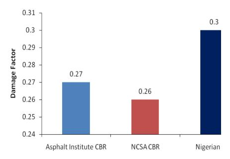
Figure 4a. CBR methods and fatigue damage factors – Asphalt Institute model (1982).
