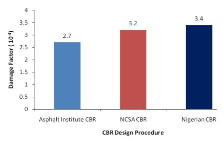
Figure 3a. CBR methods and fatigue damage factors – Heukelom and Klomp model (1962).
