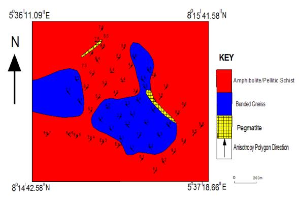
Figure 19. The geological map produced from the superposition of the anisotropy directions and the resistivity map of Odo Ara.
