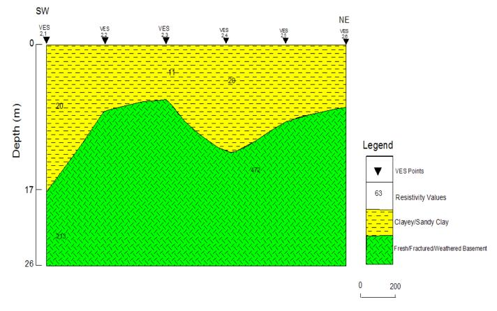
Figure 14. The geoelectric section for profile 2 of the study area.
