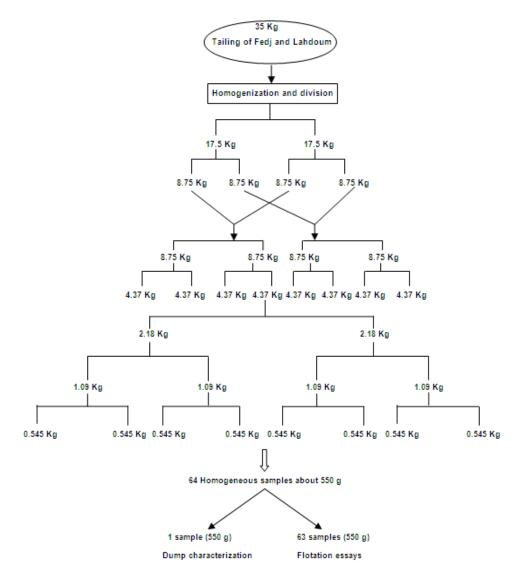
Figure 6. Representative samples through the homogenization and quartering.
