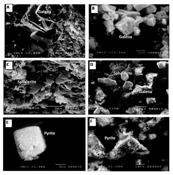
**Figure 12.** SEM images of cubic galena, sphalerite and pyrite in Fedj Lahdoum tailings (A): Galena (20  $\mu$ m) in its cubic form in a sphalerite sample (30  $\mu$ m). (B): Free galena grains (2  $\mu$ m). (C): Free sphalerite (5  $\mu$ m). (D): Mixed grain of galena-sphalerite (50  $\mu$ m). (E): Free pyrite grain (20  $\mu$ m). (F): Free pyrite graine (30  $\mu$ m).
