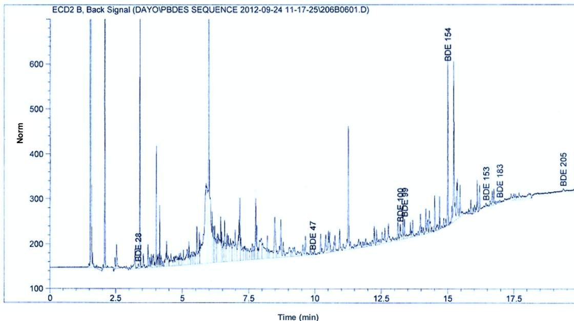
Figure 2. Chromatogram of PBDEs analysis of mid lagoon sediment sample.
