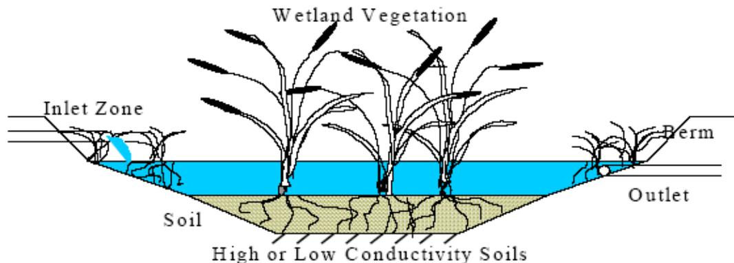
Figure 3. Free surface flow constructed wetland (Sauer and Kimber, 2001)
