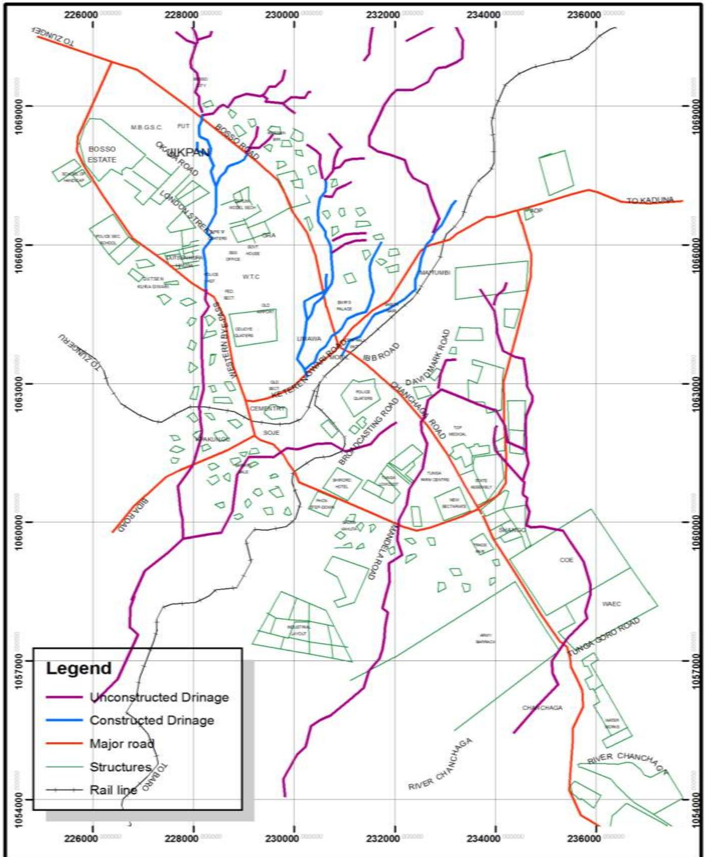
Figure 2. Constructed and unconstructed drainage channels in Minna.
