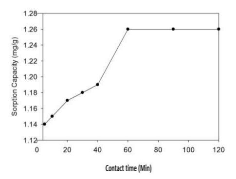
**Figure 1.** Sorption of Fluoride ion as a function of contact time initial  $F^-$  concentration of 20 mg.L<sup>-1</sup>, *Moringa* dosage of 2 g, volume of test solution 250 ml, pH ±7 and contact time 5 to 120 min.
