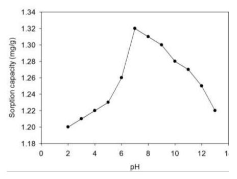
**Figure 2.** Effects of pH on fluoride ion sorption capacity of *M. stenopetala* seeds , initial fluoride ion concentration of 10 mg.L<sup>-1</sup>, *Moringa* dosage 2 g, volume of test solution 250 ml, contact time 60 min.
