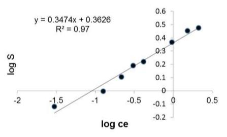
**Figure 6.** Freundlich isotherm for adsorption of Fluoride ion, initial Fluoride ion concentration 0 to 40 mg.  $L^{-1}$ , *Moringa* dosage 2 g, volume of test solution 250 ml, pH ±7, contact time 60 min.
