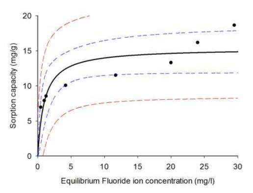
**Figure 8.** Binding of fluoride ion on *Moringa stenopetala* powder, initial fluoride ion concentration 0 to 40 mg. L<sup>-1</sup>, *Moringa* dosage 2 g, pH  $\pm$ 7, volume of test solution 250 ml, contact time 60 minutes. Solid line = Sorption capacity vs. Equilibrium fluoride ion concentration; black dots = Sorption capacity vs. Equilibrium fluoride ion concentration; Short-Short line = 95% confidence band; Medium dash line = 95% prediction band.
