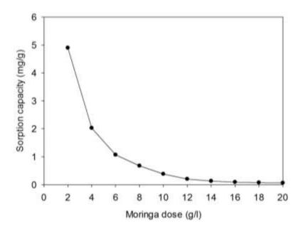
**Figure 4.** Sorption of capacity of Fluoride ion at different dosage of *Moringa*, initial concentration 10 mg.L<sup>-1</sup>, pH  $\pm$ 7, volume of test solution 250 ml, contact time 60 min.
