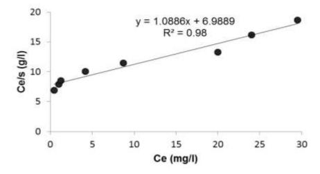
**Figure 7.** Langmuir Isotherm for adsorption of fluoride ion, initial Fluoride concentration 0 to 40 mg.  $L^{-1}$ , *Moringa* dosage 2 g, pH ±7, volume of test solution 250 ml, contact time 60 min.
