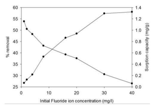
**Figure 3.** Effects of initial Fluoride ion concentration on biosorption by *M. stenopetala*, initial fluoride ion concentration 0 to 40 mg.  $L^{-1}$ , *Moringa* dosage 2 g, volume of test solution 250 ml, pH ±7, contact time 60 min.
