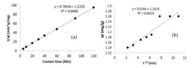
**Figure 5.** Plot of pseudo-second-order model (a) and Intraparticle diffusion model (b) for fluoride ion adsorption onto *Moringa* powder. Initial Fluoride ion concentration 20 mg.  $L^{-1}$ , *Moringa* dosage 2 g, volume of test solution 250 ml, pH ±7.
