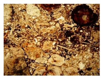
Figure 4. Thin section of OG2 at x20 (showing granular form with shell fragments)
