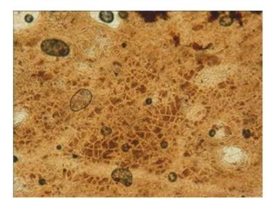
Figure 2. Thin section of nodular phosphorite (OG1 at x50).
