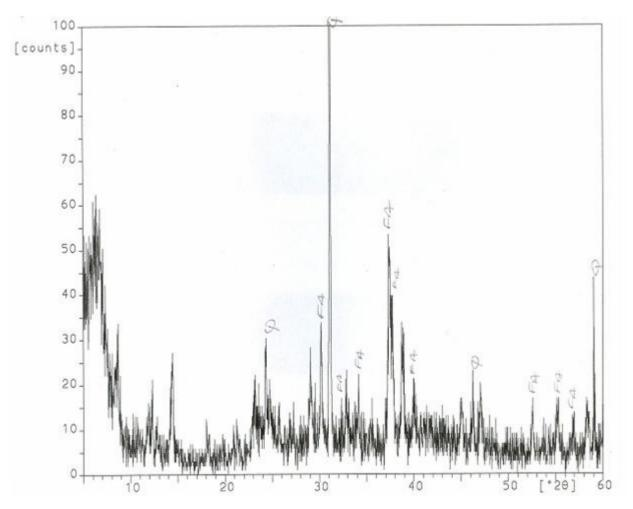
Figure 10. X - Ray diffractogram of OGMIX. FA = Flourapatite, Q = Quartz, CA - Calcite
