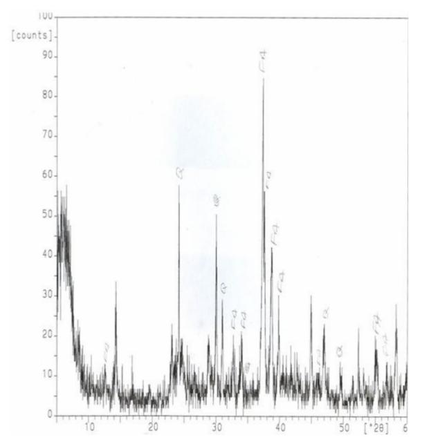
Figure 7. X – Ray diffractogram of OG2. FA = Flourapatite, Q = Quartz CA – Calcite.
