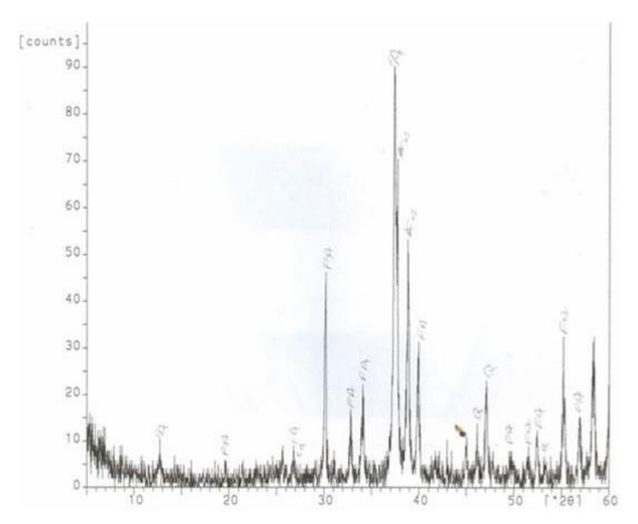
Figure 6. X – Ray diffractogram of OG1. FA = Flourapatite, Q = Quartz CA – Calcite.
