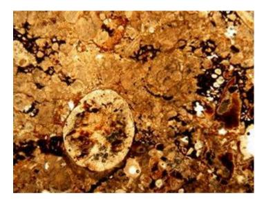
Figure 5. Thin sections of OG4 x 20 (showing granular form of Phosphorites with burrows)
