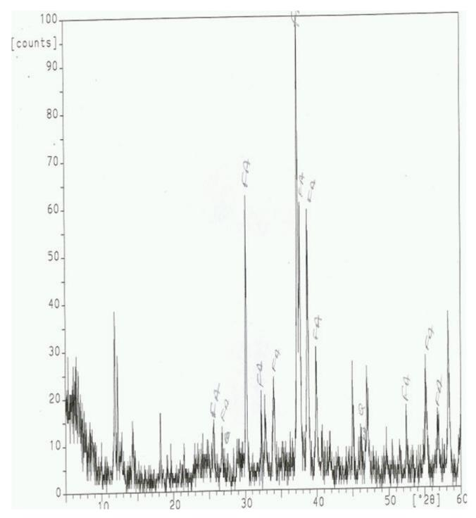
Figure 8. X – Ray diffractogram of OG3. FA = Flourapatite, Q = Quartz, CA= Calcite.
