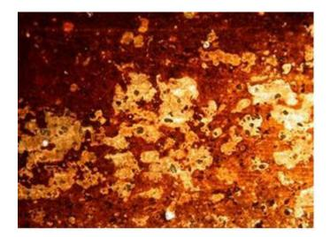
Figure 3. Thin section of Nodular Phosphorite OG  $3 \times 20$  showing Geopedal texture with Fe staining.
