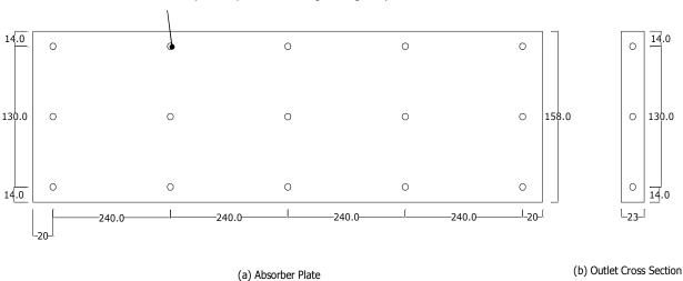
15 Nos thermocouples at equal distance along the length of plate
