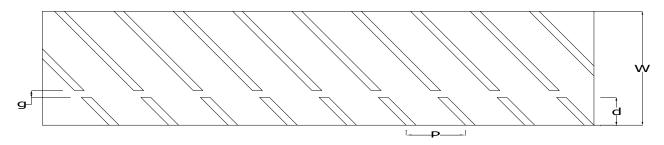
Figure 1. Geometry of 60° inclined discrete rib roughness.
