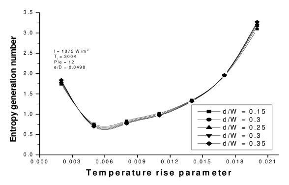
Figure 18. Entropy generation number Vs temperature rise parameter for P/e= 12 and e/D=0.0498.  $\Delta T / I$ .
