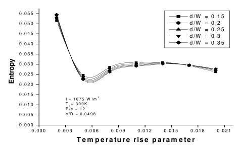
Figure 17. Entropy Vs temperature rise parameter for P/e= 12 and e/D=0.0498.
