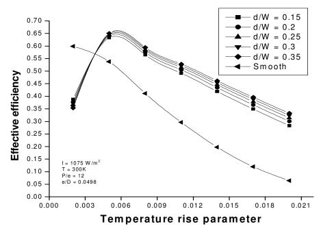
Figure 16. Effective efficiency Vs temperature rise parameter for P/e= 12 and e/D=0.0498.
