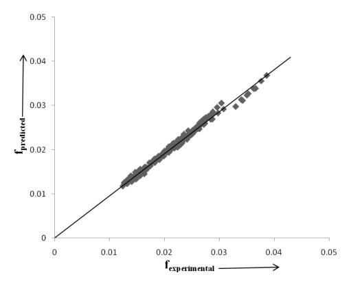
Figure 9. Comparison of friction factor for experimental values with predicted values.
