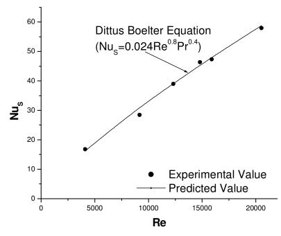
Figure 7. Nusselt number vs. Reynolds number for smooth duct.
