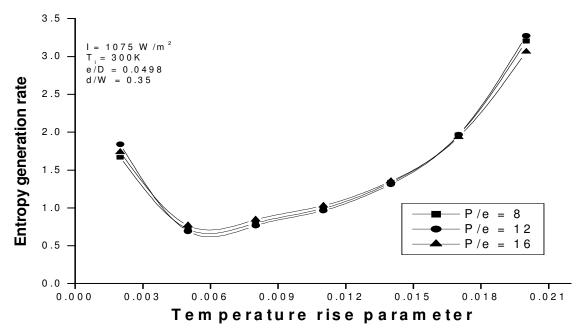
Figure 12. Entropy generation number Vs temperature rise parameter for e/D= 0.0498 and d/W=0.35.
