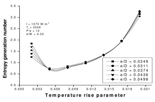
Figure 15. Entropy generation number Vs temperature rise parameter for P/e= 12 and d/W=0.35.
