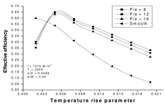
Figure 10. Effective efficiency Vs temperature rise parameter for e/D = 0.0498 and d/W = 0.35.
