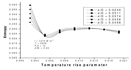
Figure 14. Entropy Vs temperature rise parameter for P/e= 12 and d/W=0.35.
