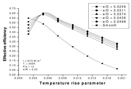
Figure 13. Effective efficiency Vs temperature rise parameter for P/e= 12 and d/W=0.35.
