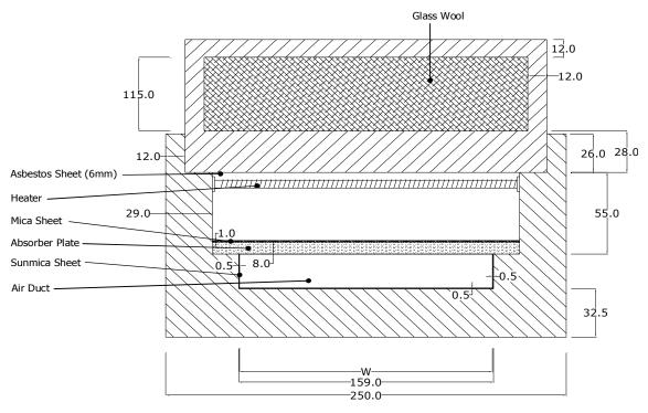
Figure 4. Cross sectional details of test section.
