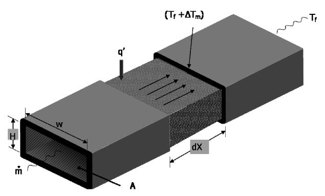
Figure 2. Forced convection heat transfer inside duct of a solar air heater.
