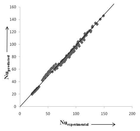
Figure 8. Comparison of Nusselt number for experimental values with predicted values.
