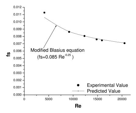
Figure 6. Friction factor vs. Reynolds number for smooth duct.
