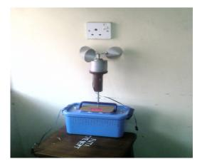
Figure 5. Pictorial view of the developed cup anemometer.
