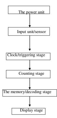
**Figure 1.** Design flowchart of the digital electronic system.
