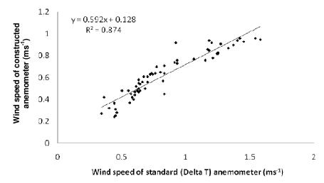
**Figure 6.** Calibration curve 1 showing the relationship between constructed and standard cup anemometer.
