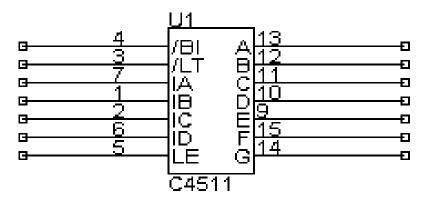
Figure 4. Pin configuration of 4511B latch/decoder.
