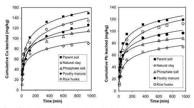
Figure 3. Cumulative Cu and Pb kinetically extracted with 0.05 M EDTA in the parent soil and its sub-samples amended (at 20% w/w) with different immobilizing agents.
