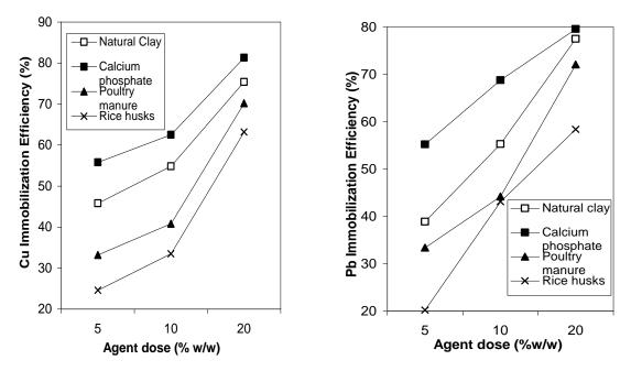
Figure 1. Efficiency of Cu and Pb immobilization in soil amended with different agents.
