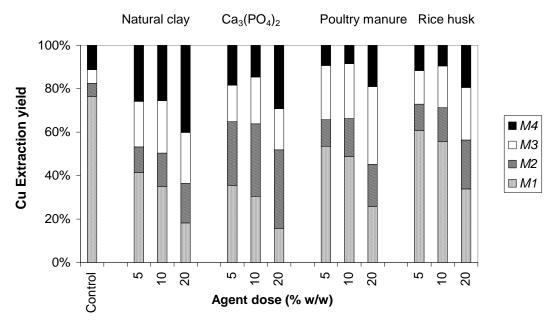
**Figure 2a.** Extraction yields (%) of Cu in operationally defined pools of contaminated soil amended with different immobilizing agents extracted by the BCR sequential procedure.
