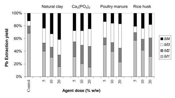
**Figure 2b.** Extraction yields (%) of Pb in operationally defined pools of contaminated soil amended with different immobilizing agents extracted by the BCR sequential procedure.
