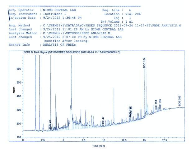
Figure 2. Chromatogram of PBDEs analysis of mid lagoon sediment sample.
