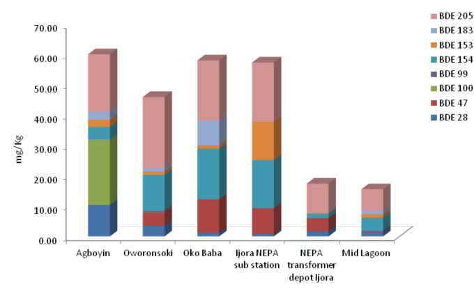
Figure 3. Mean value for PBDE congeners analyzed in sediment between June 2011 and July 2012.
