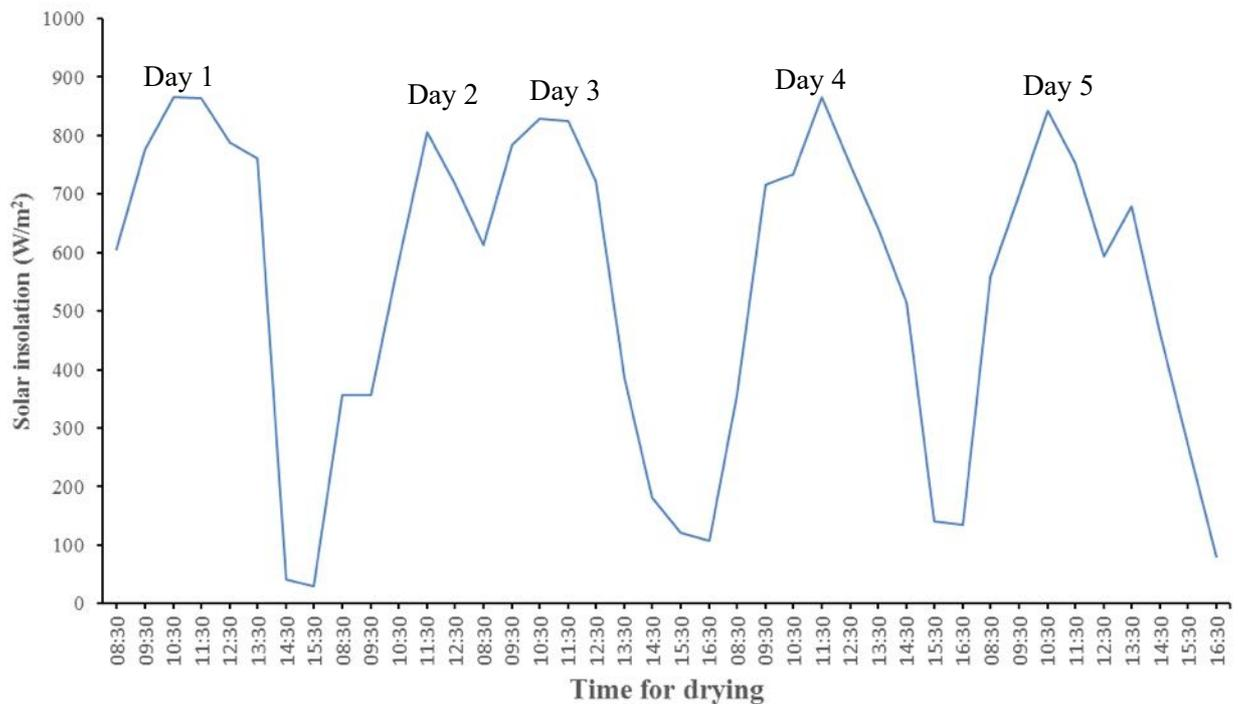
**Figure 4: Solar insolation trend during solar drying**
