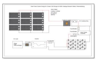
(C) SPV system for the cooling
