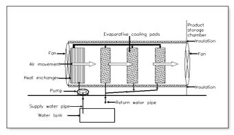
(B) Schematic diagram of storage chamber (C)
