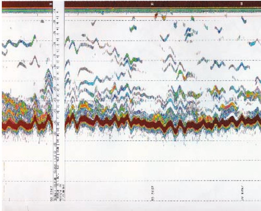
Fig. 2: *Sv* echogram at 38 kHz recorded using the submersible transducer in October 1998. The ensonified Cape horse mackerel were aggregated near the bottom (120 m) during this experiment
