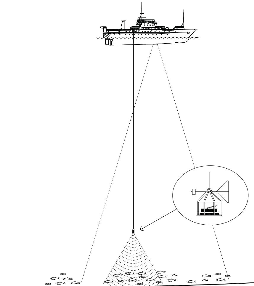
Fig. 1: Experimental set-up during the target strength measurements, showing the acoustic beams of the hull-mounted and the submersible transducers. The steel housing of the submersible transducer is enlarged
