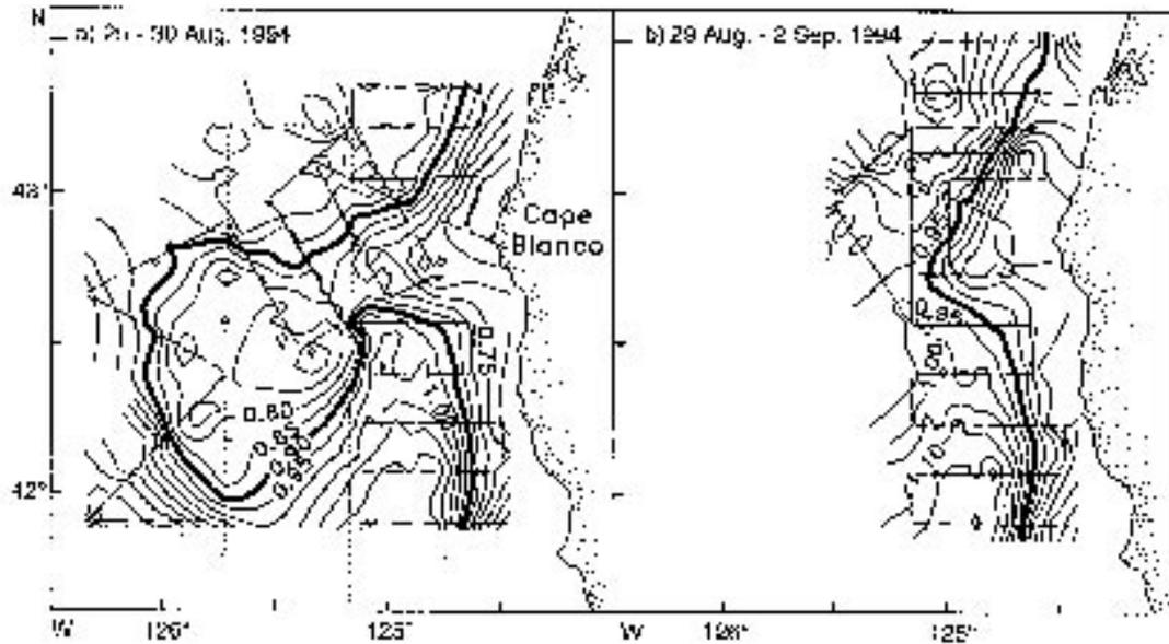
Fig. 2: Contour maps of geopotential anomaly (dynamic height in meters multiplied by the acceleration of gravity) at 23 m relative to 55 m from SeaSoar surveys during (a) 25–30 August 1994 and (b) 29 August–2 September 1994. Individual CTD depth profiles are denoted by dots along the ship's track and the  $0.9 \text{ m}^2\text{s}^{-2}$  geopotential anomaly contour is highlighted to emphasize the pinching-off of a counter-clockwise (cyclonic) eddy off Cape Blanco, Oregon
