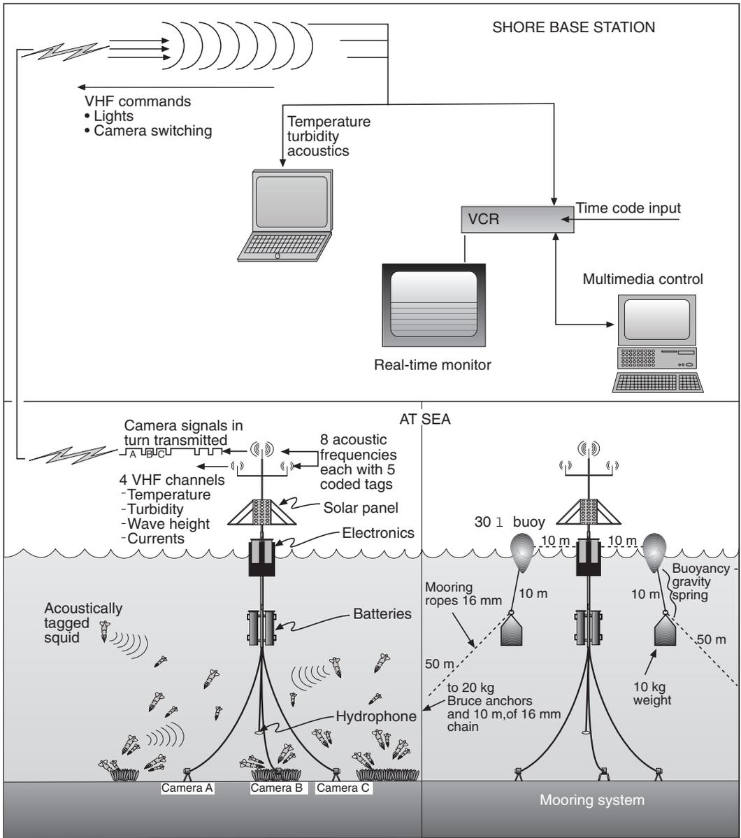
Fig. 9: Schematic diagram showing the main components of the hardware designed and constructed to quantify squid spawning behaviour and environmental influences
