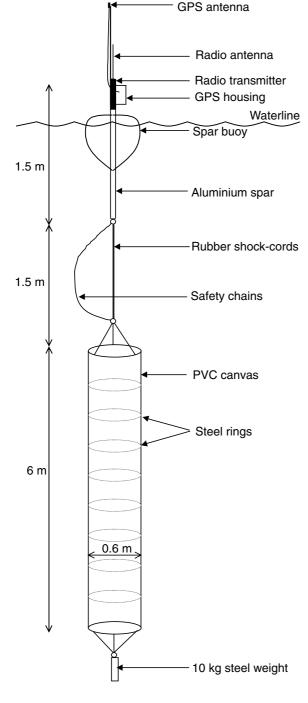
Fig. 1: Diagrammatic view of the holey-sock drogue. Not shown are the 20-cm diameter holes cut into the PVC canvass
