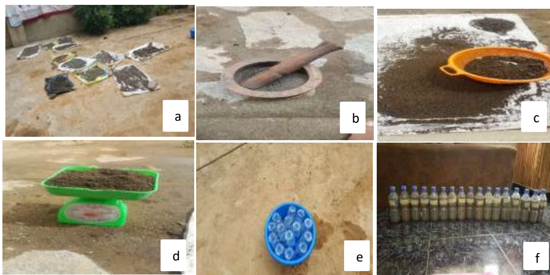
Figure 3: Sample Preparation Process (a) Drying (b) Pulverization using Grinder (c) Sieving (d) Weighing (e) Cleaned Container (f) Samples in Temporary Container
