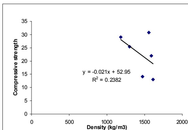
Figure 6: Correlation between Density and Compressive Strength
