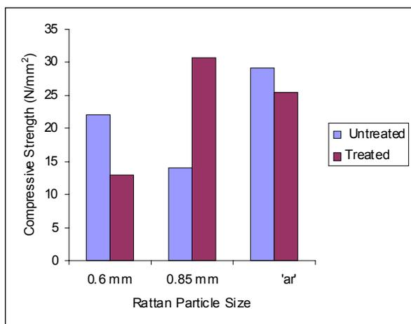
Figure 5: Effects of Particle Size and CaCl<sub>2</sub> on Compressive Strength
