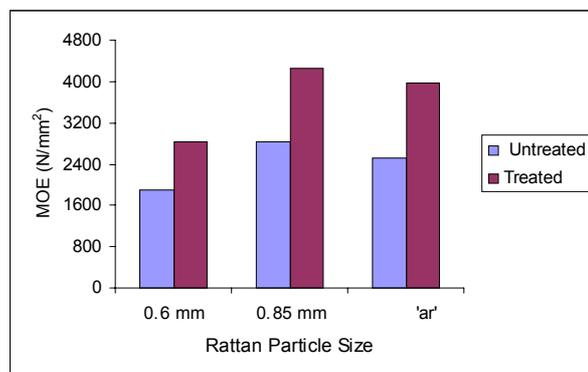
Figure 2: Effects of Particle Size and CaCl<sub>2</sub> on MOE
