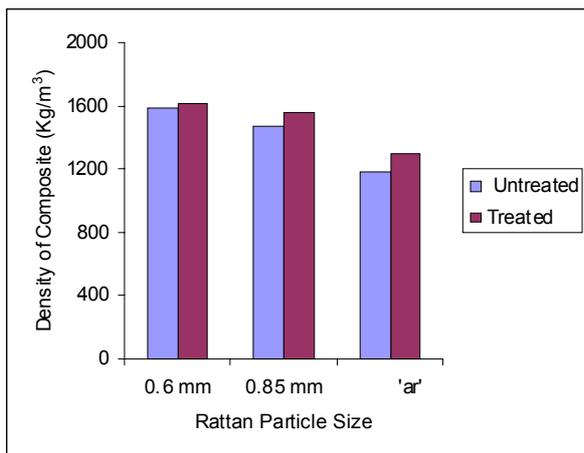
Figure 1: Effects of Particle Size and CaCl<sub>2</sub> on the Density
