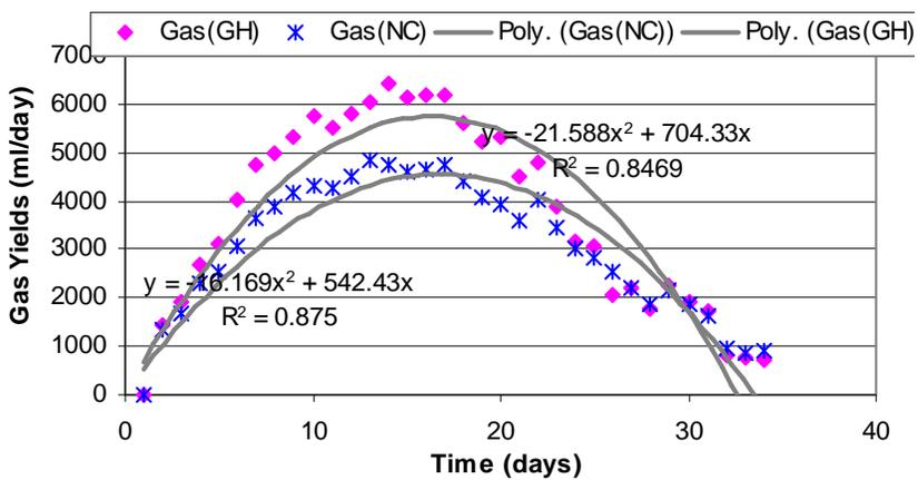
Figure 4: Plots of gas yields and polynomial equations for the corresponding time under GH and conditions NC
