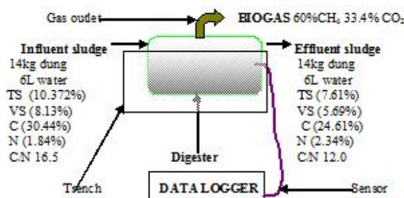
Figure 1: Experimental setup of biogas plant
