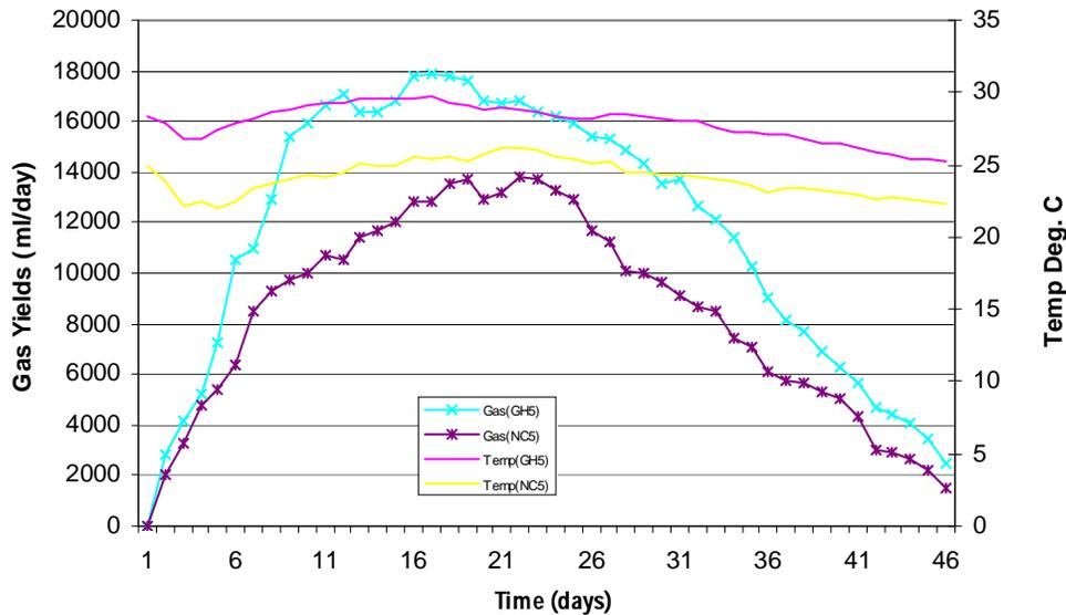
Figure 6: Plots of gas yields and temperature for the corresponding time of under GH and NC
