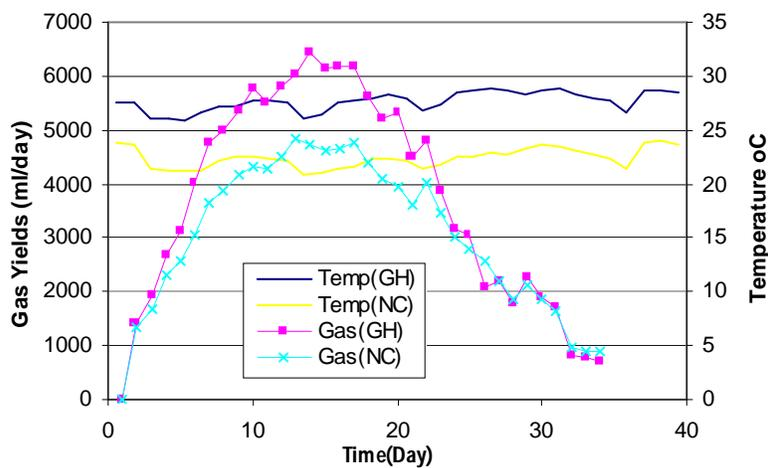
Figure 3: Temporal volumetric gas yields and digester temperature under greenhouse (GH) and natural condition (NC)
