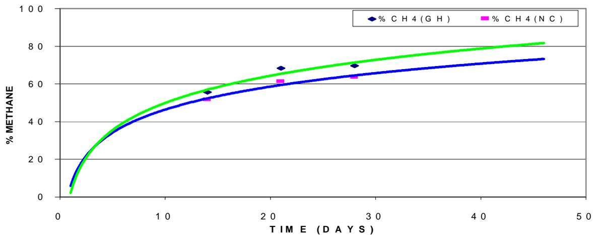
Figure 2: Daily variation of methane in biogas under GH and NC
