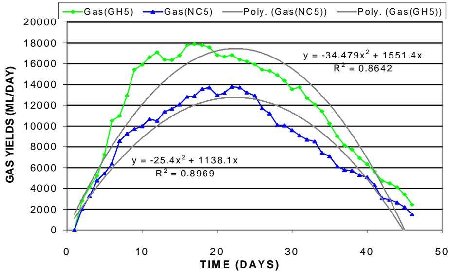
Figure 5: Plots of gas yields and polynomial equations for the corresponding time under GH and NC
