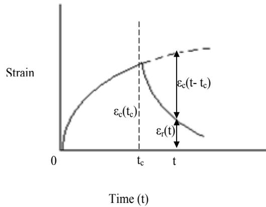
**Figure 1: Typical Creep and Recovery Behaviour (Crawford, 2005)**
