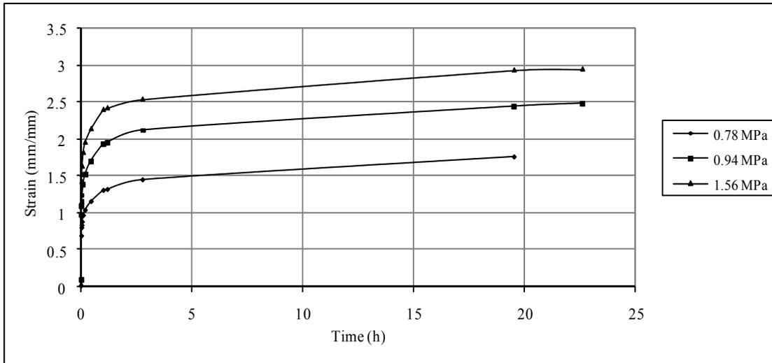
Figure 2 (c): Constant Temperature Creep Curves at 50°C
