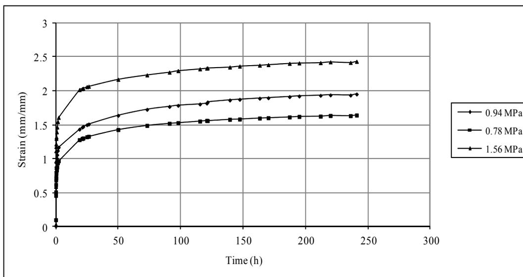
Figure 2 (b): Constant Temperature Creep Curves at 40°C
