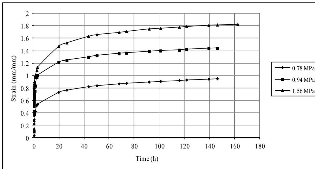
Figure 2 (a): Constant Temperature Creep Curves at 30°C
