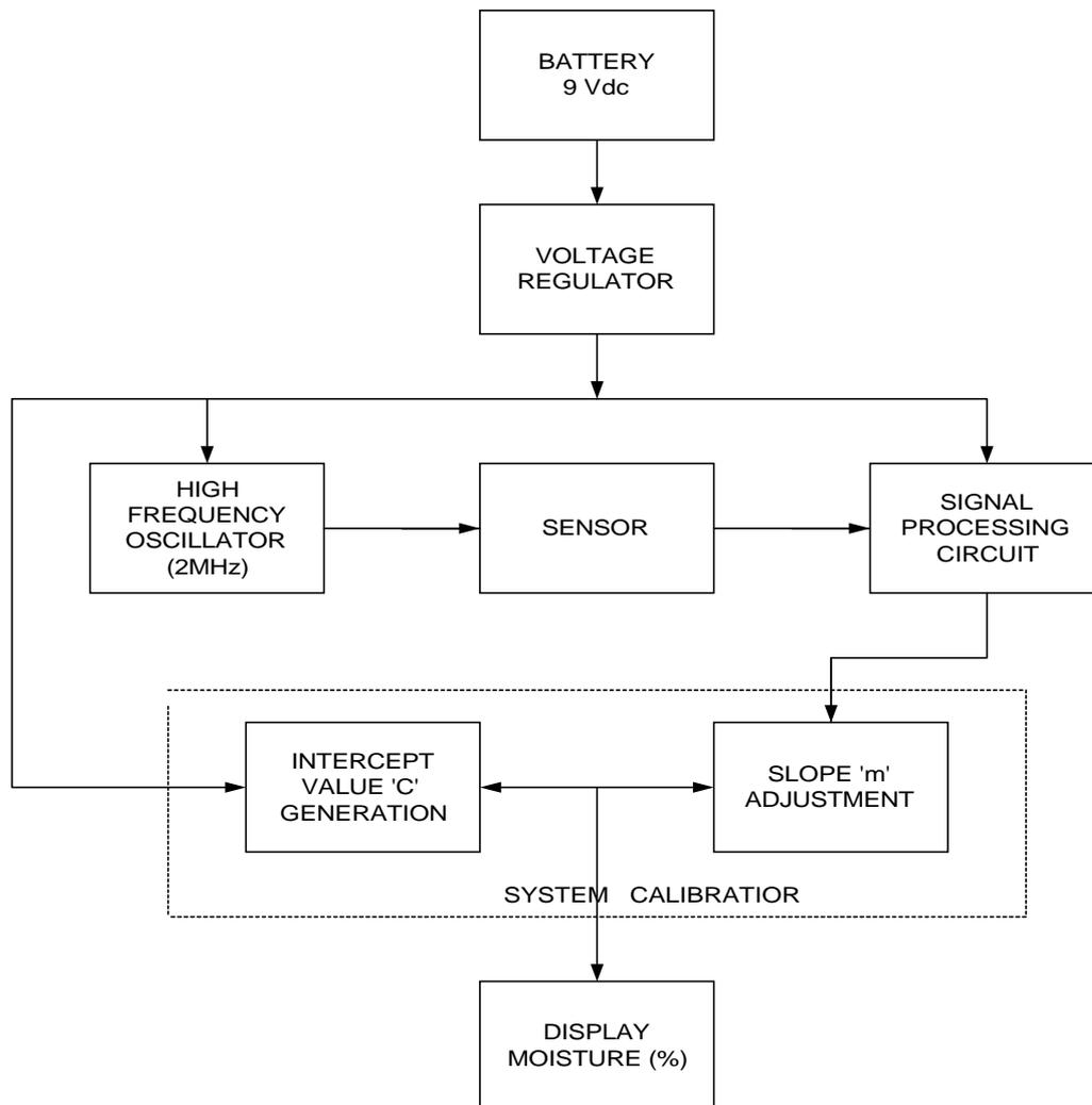
Figure 1: Functional Block Diagram of the capacitance-based moisture meter
