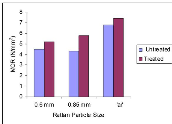
Figure 3: Effects of Particle Size and CaCl<sub>2</sub> on MOR
