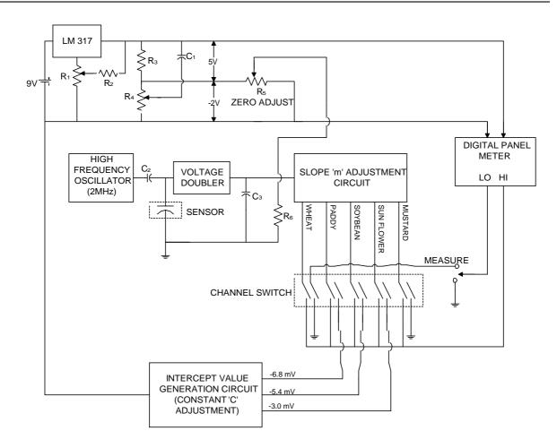
Figure 2: The electronic circuit of the grain moisture meter
