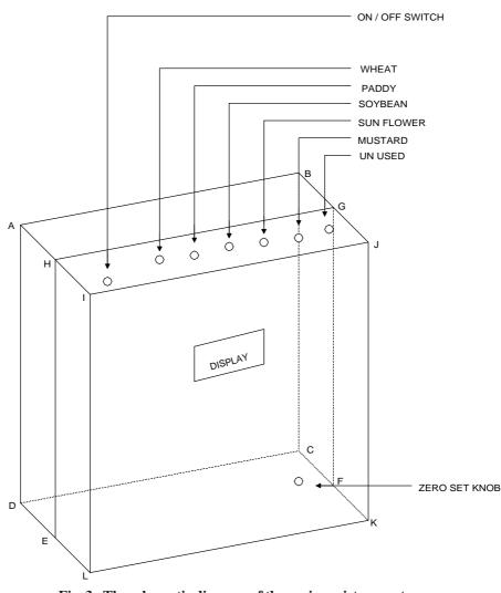
Fig. 3: The schematic diagram of the grain moisture meter
