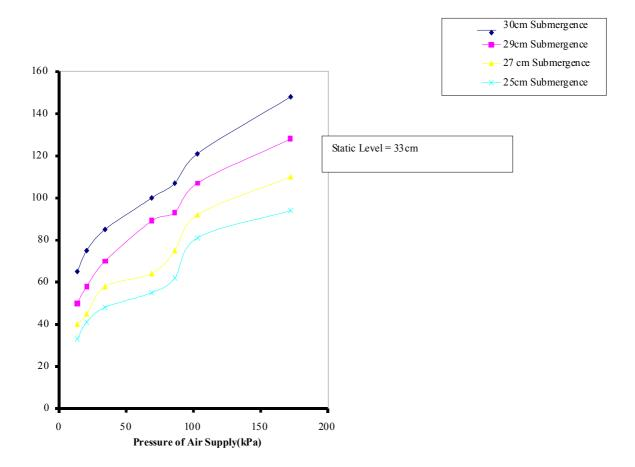
Figure 4: Plot of Water Lift against Air Supply Presure in Sand-Water Medium
