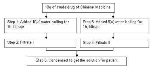
Figure 2: Flowchart of the conventional extraction method
