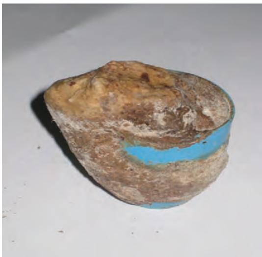
**Fig. 4:** The plastic bottle cap covered by phosphatic encrustations after its extraction.
