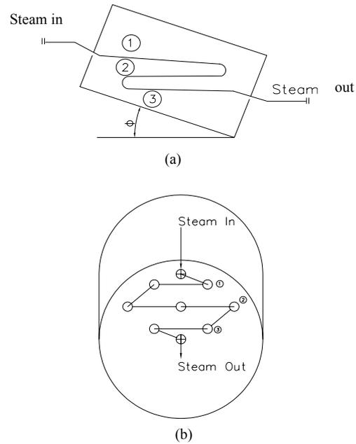
**Figure 3 (a) and (b): The heating tube arrangement**
