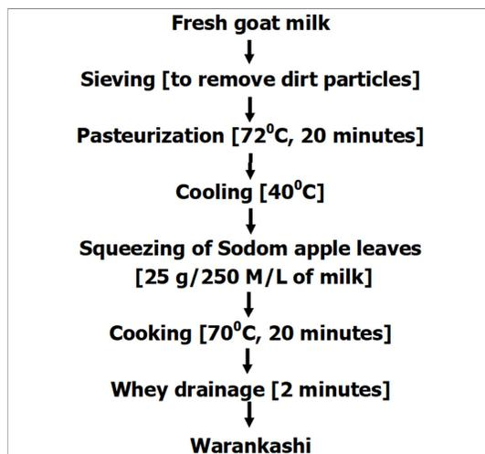
**Figure 1:** The flow diagram for cheese production (modified from Adetunji and Babalobi, 2011)
