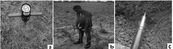
Figure 2: Measurement of soil resistances (Compact model n° 6120 (a), use of the compactometer (b), measurement with a pocket penetrometer (c))
