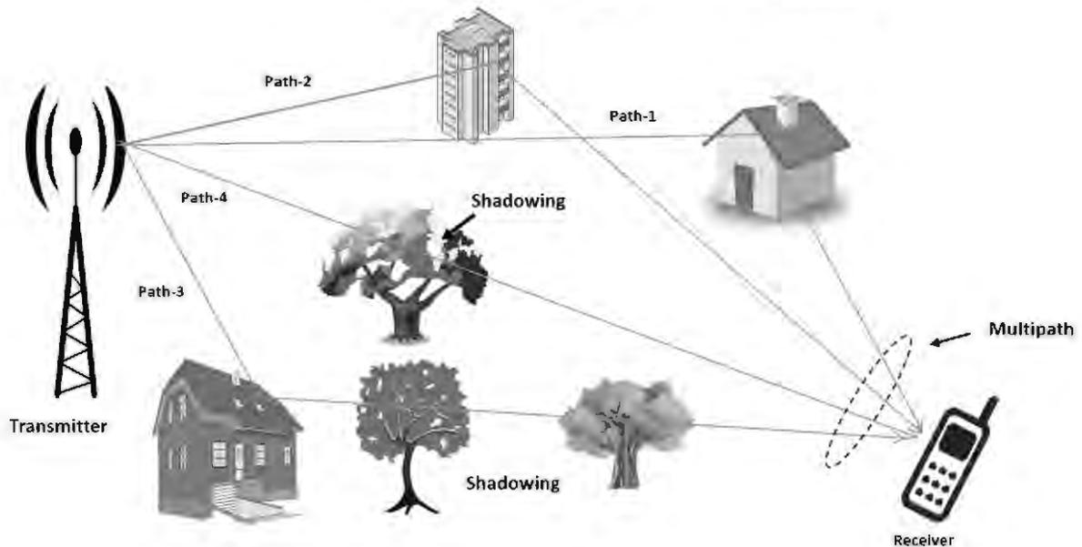
Figure 1. Radio Propagation in Built-up Areas
