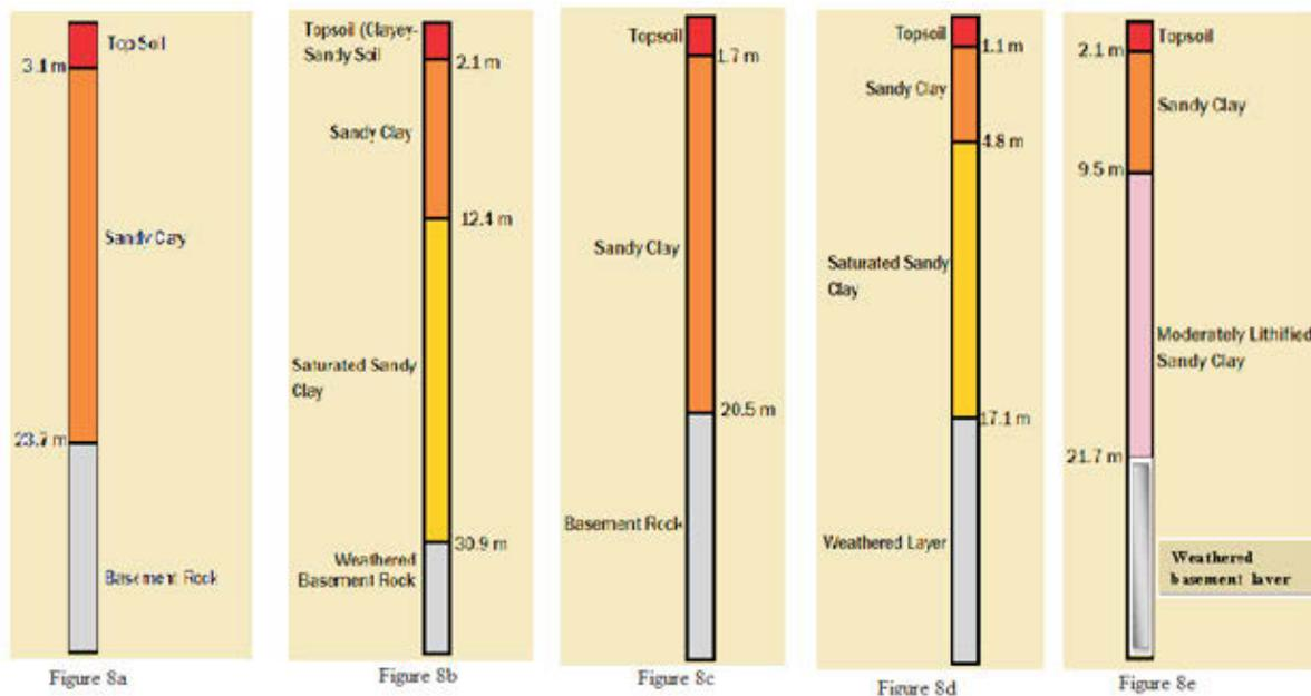
Figure 8: (a) Inferred lithology of VES 1, (b) Inferred lithology of VES 2, (c) Inferred lithology of VES 3, (d) Inferred lithology of VES 4, (e) Inferred lithology of VES 5.
