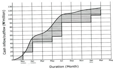
Figure 2. S-Curve for First Extension Project at FCE, Zaria
