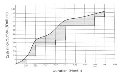
Figure 3. S-Curve for the Second Extension Project at FCE, Zaria
