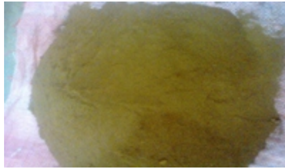
Plate I: Volcanic ash sieved to 75 \mu m
