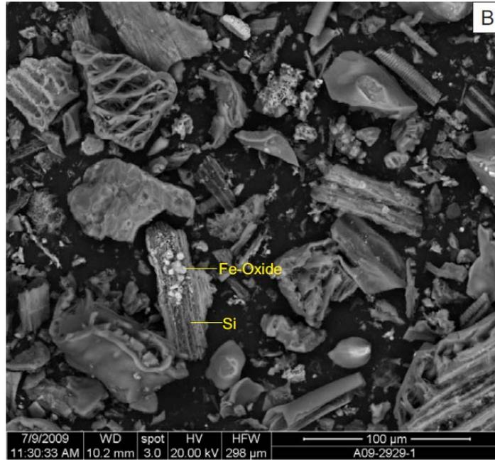
Plate I: Microstructure of the milled RHA ( $\times 1000$ ).
