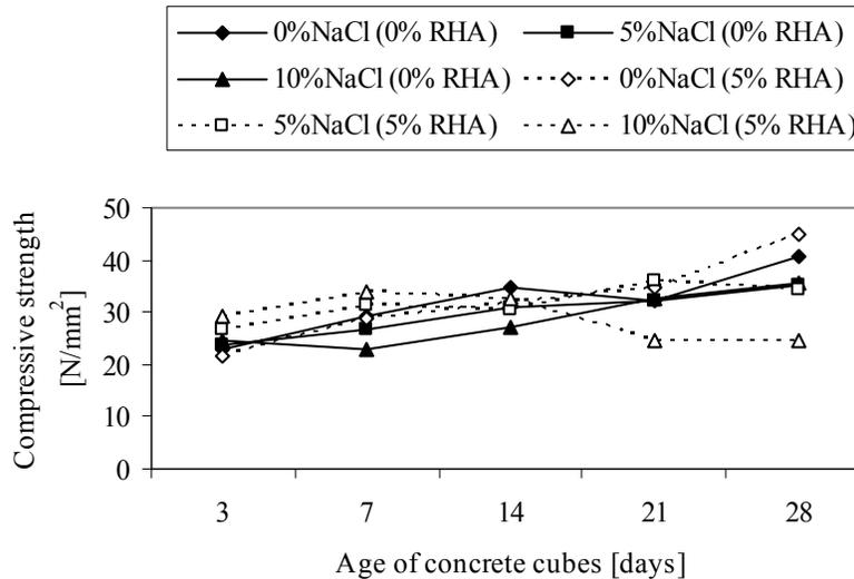
Figure 3: Effect of sodium chloride solutions of compressive strength of concrete.
