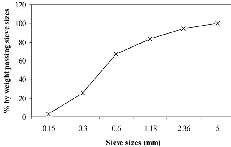
Figure 1: Particle size distribution of fine aggregates.
