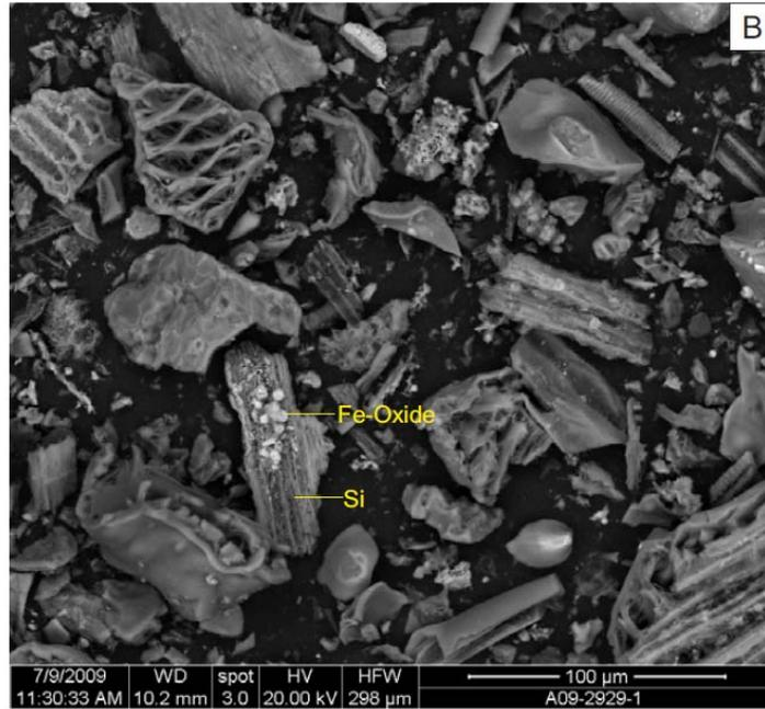
Plate I: Microstructure of the milled RHA ( $\times 1000$ ).
