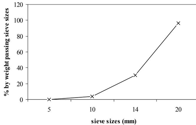
Figure 2: Particle size distribution of coarse aggregates.
