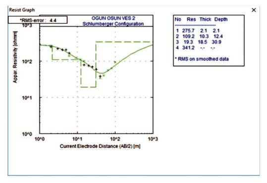
Figure 4: Interpreted Schlumberger depth sounding curve for VES 2.
