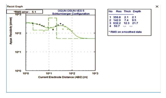
Figure 7: Interpreted Schlumberger depth sounding curve for VES 5
