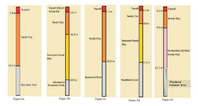
Figure 8: (a) Inferred lithology of VES 1, (b) Inferred lithology of VES 2, (c) Inferred lithology of VES 3,(d) Inferred lithology of VES 4,(e) Inferred lithology of VES 5.
