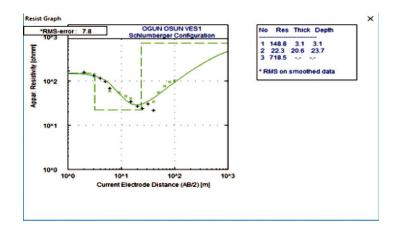
Figure 3: Interpreted Schlumberger depth sounding curve for VES 1.
