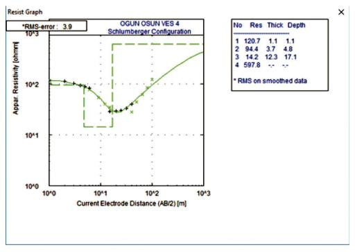
Figure 6: Interpreted Schlumberger depth sounding curve for VES 4
