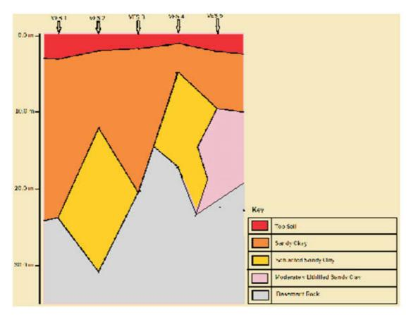
Figure 9: The Geoelectric section of the VES.
