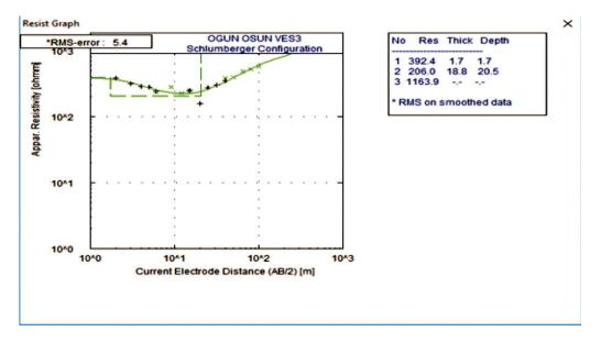
Figure 5: Interpreted Schlumberger depth sounding curve for VES 3
