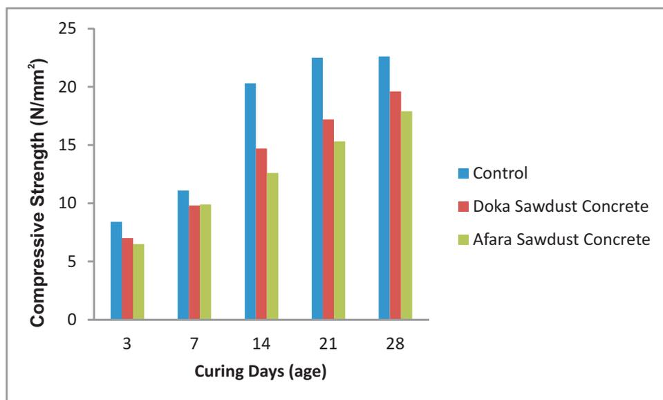
**Figure 1. Compressive strength of the Concrete Samples**
