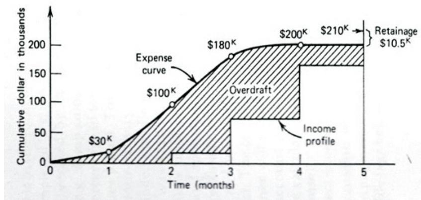
Figure 1: Typical S-Curve
