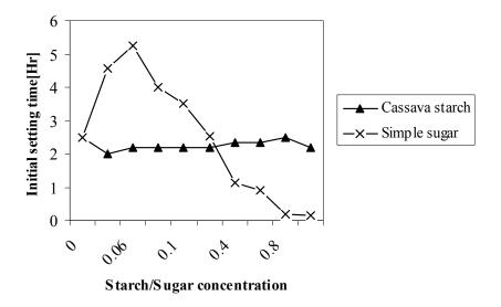
Figure 5. Effects of cassava starch and sugar on initial setting time of cement mortar.
