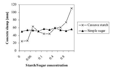
Figure 6. Effect of cassava starch and sugar on slump of fresh concrete.
