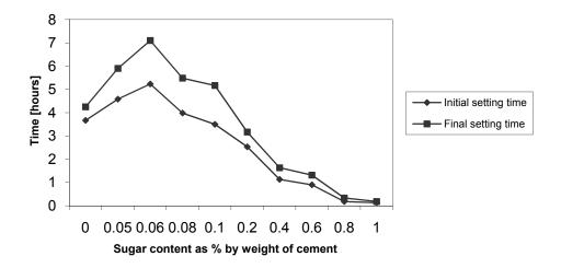
Figure 3. Effect of sugar on setting time of cement mortar.
