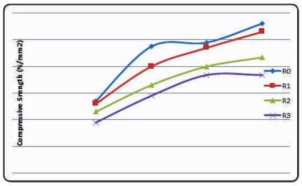
Figure 2: Compressive strength of Brick Sample Made with Various % Partial Replacements of Cement with WA
