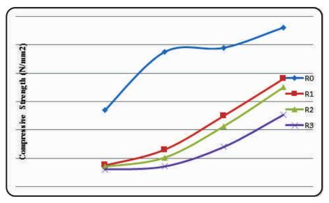
Figure 1: Compressive strength of brick sample made with various % partial replacements of cement with RHA
