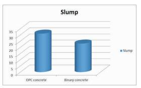
Figure 1: Slump of OPC Concrete and Binary Concrete
